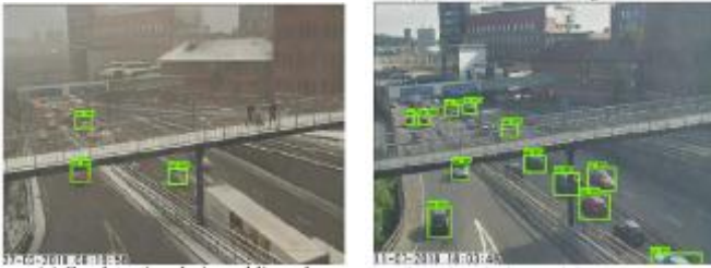
(a) Car detection during a blizzard (b) Car detection during rush hour on a summer day
