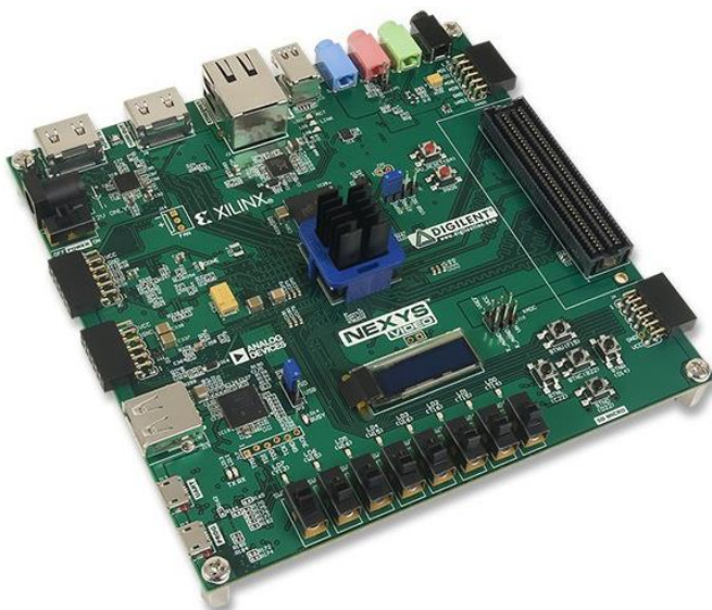
Fig. 13.4 – General view of the Nexys Video Artix-7 FPGA module [16]
