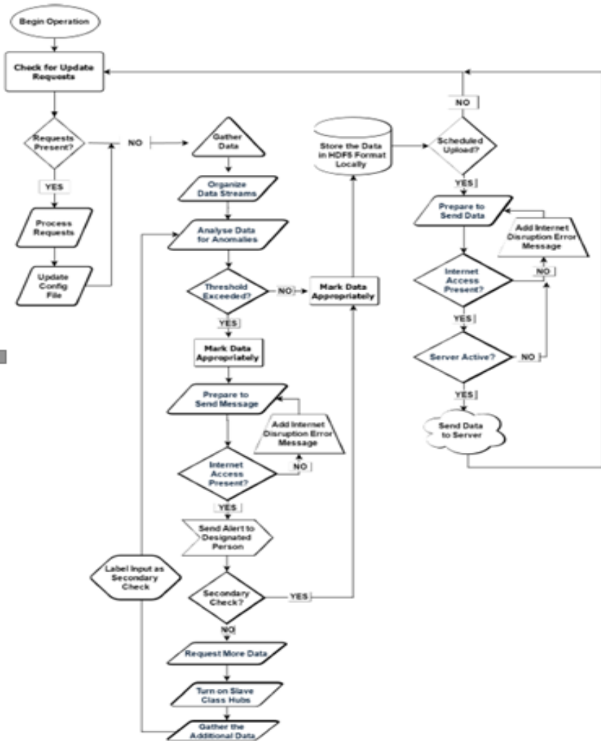
Fig. 14.5 - A diagram displaying the high level algorithm of autonomous modes of operation
