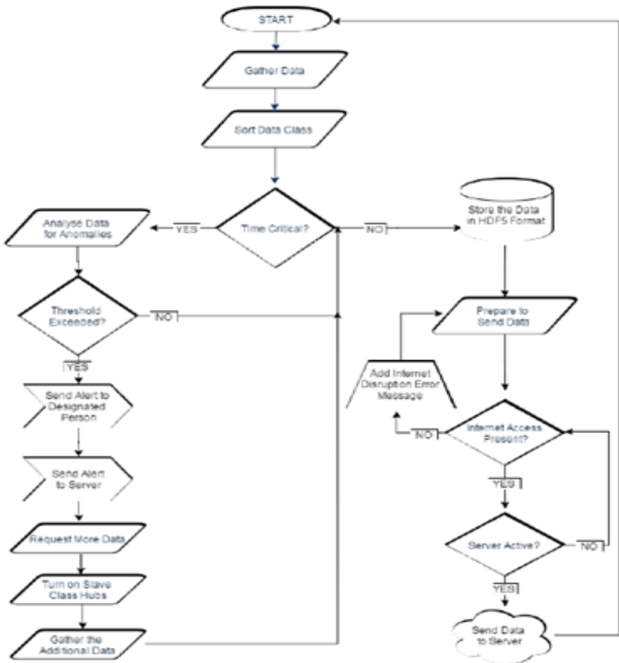
Fig. 14.6 - A diagram displaying the high level algorithm of semi-autonomous modes of operation
